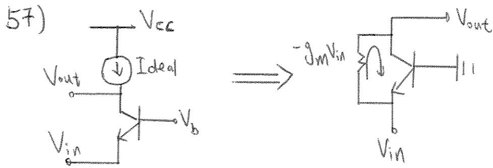
Since an ideal current source is an open circuit, the signal current produced by the transistor has no where to go but  $V_o$ .
