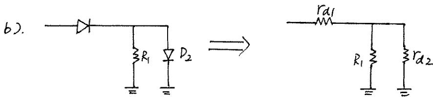
$$R_{in} = r_{d1} + R_1 \parallel r_{d2} \quad (\text{// means in parallel})$$
