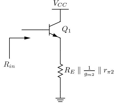
$$R_{in} = \boxed{r_{\pi 1} + (1 + \beta_1) \left( R_E \parallel \frac{1}{g_{m2}} \parallel r_{\pi 2} \right)}$$
