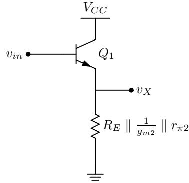
$$\frac{v_X}{v_{in}} = \frac{R_E \parallel \frac{1}{g_{m2}} \parallel r_{\pi 2}}{\frac{1}{g_{m1}} + E \parallel \frac{1}{g_{m2}} \parallel r_{\pi 2}}$$
