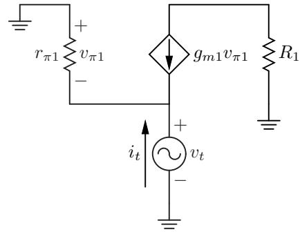
$$i_t = -\frac{v_{\pi 1}}{r_{\pi 1}} - g_{m1}v_{\pi 1}$$
