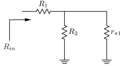
$$R_{in} = \boxed{R_1 + R_2 \parallel r_{\pi 1}}$$
