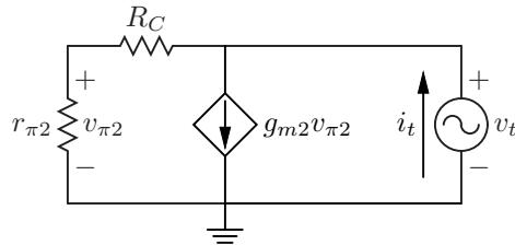
$$\begin{aligned} i_t &= g_{m2}v_{\pi2} + \frac{v_{\pi2}}{r_{\pi2}} \\ v_{\pi2} &= \frac{r_{\pi2}}{r_{\pi2}+R_C}v_t \\ i_t &= \left(g_{m2}+\frac{1}{r_{\pi2}}\right)\frac{r_{\pi2}}{r_{\pi2}+R_C}v_t \\ R_{out} &= \frac{v_t}{i_t} \\ &= \boxed{\left(\frac{1}{g_{m2}}\parallel r_{\pi2}\right)\frac{r_{\pi2}+R_C}{r_{\pi2}}} \end{aligned}$$
