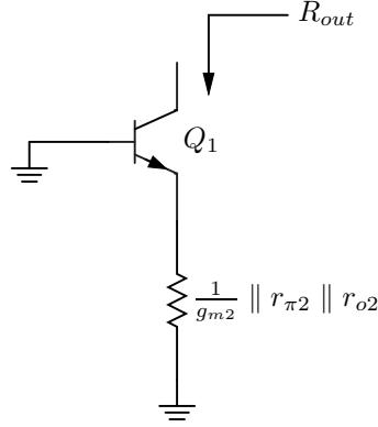
$$R_{out} = \boxed{r_{o1} + (1 + g_{m1}r_{o1}) \left( r_{\pi1} \parallel \frac{1}{g_{m2}} \parallel r_{\pi2} \parallel r_{o2} \right)}$$
