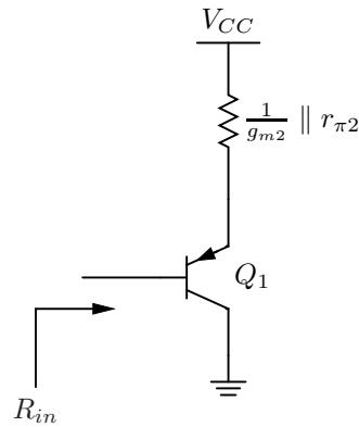
$$R_{in} = \boxed{r_{\pi 1} + (1 + \beta_1) \left( \frac{1}{g_{m2}} \parallel r_{\pi 2} \right)}$$
