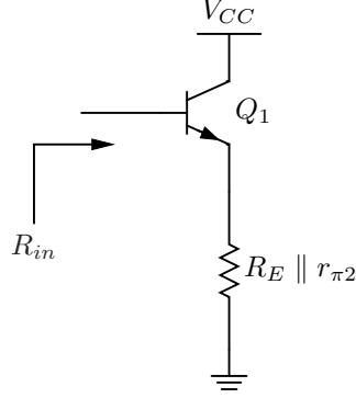
$$R_{in} = \boxed{r_{\pi 1} + (1 + \beta_1)(R_E \parallel r_{o1})}$$
