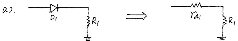
$$R_{in} = r_{d1} + R_1$$
