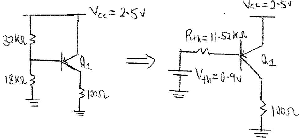
$$I_c = \beta_{PNP} \left( \frac{2.5 - |V_{BE}| - V_{th}}{R_{th}} \right)$$
