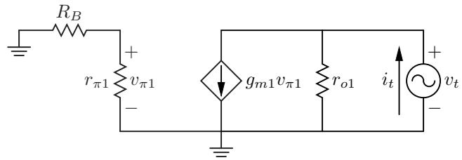
$$i_t = g_{m1}v_{\pi1} + \frac{v_t}{r_{o1}}$$
