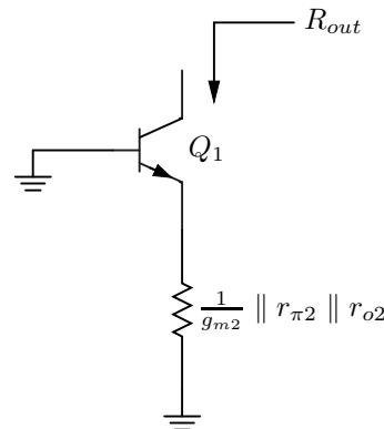
$$R_{out} = [r_{o1} + (1 + g_{m1}r_{o1}) \left( r_{\pi1} \parallel \frac{1}{g_{m2}} \parallel r_{\pi2} \parallel r_{o2} \right)]$$
