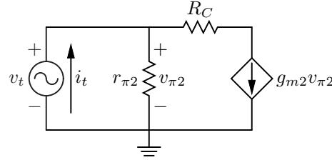
$$i_t = \frac{v_{\pi2}}{r_{\pi2}} + g_{m2}v_{\pi2}$$
