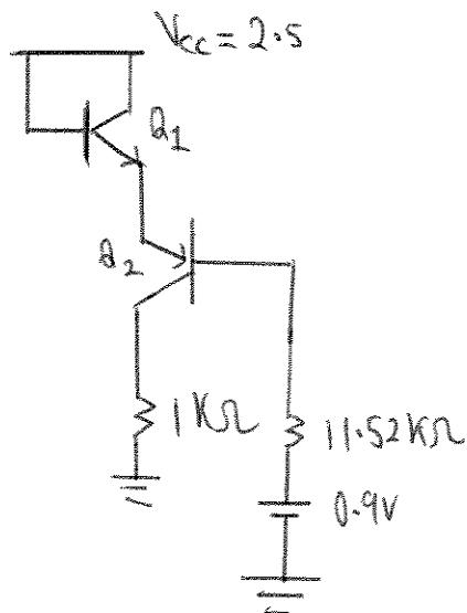
$$I_{c2} = \frac{[2.5 - (V_{BE1} + V_{BE2}) - 0.9]50}{11.52K}$$
