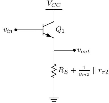
$$A_v = \frac{R_E + \frac{1}{g_{m2}} \parallel r_{\pi 2}}{\frac{1}{g_m 1} + R_E + \frac{1}{g_{m2}} \parallel r_{\pi 2}}$$
