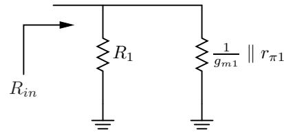
$$R_{in} = \boxed{R_1 \parallel \frac{1}{g_{m1}} \parallel r_{\pi 1}}$$
