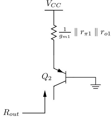
$$R_{out} = \boxed{r_{o2} + (1 + g_{m2}r_{o2}) \left( r_{\pi 2} \parallel \frac{1}{g_{m1}} \parallel r_{\pi 1} \parallel r_{o1} \right)}$$
