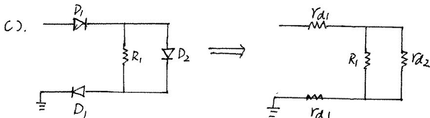
$$R_{in} = 2r_{d1} + R_1 \parallel r_{d2}$$
