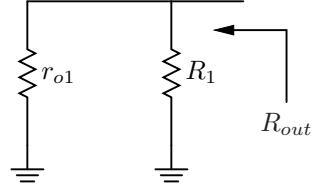
$$R_{out} = [r_{o1} \parallel R_1]$$
