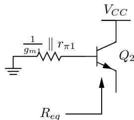
$$R_{eq} = \boxed{\frac{r_{\pi 2} + \frac{1}{g_{m1}} \parallel r_{\pi 1}}{1 + \beta_2}}$$
