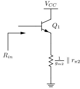
$$R_{in} = \boxed{r_{\pi 1} + (1 + \beta_1) \left( \frac{1}{g_{m2}} \parallel r_{\pi 2} \right)}$$
