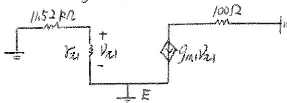
$$g_{m1} = \frac{3.67 \text{ mA}}{26 \text{ mV}} = 0.141 \text{ S}$$
