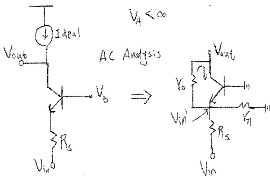
$$A_v = \frac{V_{out}}{V_{in}} = \left( \frac{V_{in}'}{V_{in}} \right) \left( \frac{V_{out}}{V_{in}'} \right), \quad \left( \frac{V_{in}'}{V_{in}} \right) = \frac{r_\pi}{r_\pi + R_s}$$
