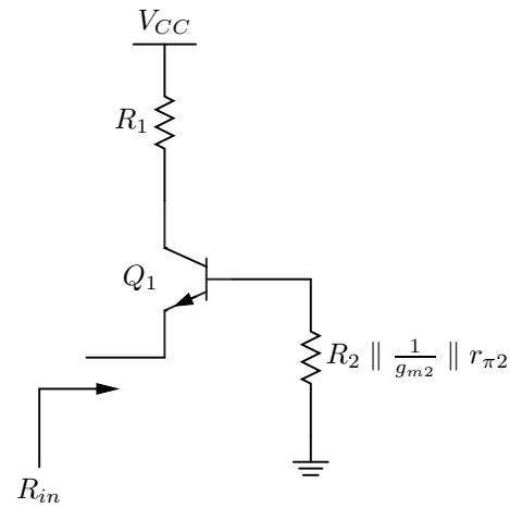
$$R_{in} = \boxed{\frac{r_{\pi 1} + R_2 \parallel \frac{1}{g_{m2}} \parallel r_{\pi 2}}{1 + \beta_1}}$$
