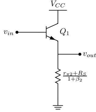
$$A_v = \frac{\frac{r_{\pi 2} + R_s}{1 + \beta_2}}{\frac{1}{g_m 1} + \frac{r_{\pi 2} + R_s}{1 + \beta_2}}$$
