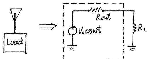
$$\text{Average power delivered to load} = (I_{rms})^2 R_L,$$
