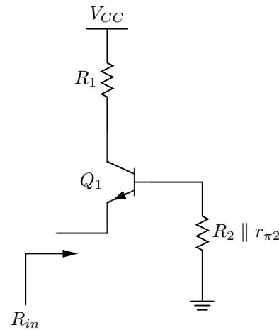
$$R_{in} = \boxed{\frac{r_{\pi 1} + R_2 \parallel r_{\pi 2}}{1 + \beta_1}}$$
