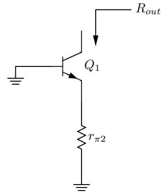
$$R_{out} = \boxed{r_{o1} + (1 + g_m r_{o1}) (r_{\pi 1} \parallel r_{\pi 2})}$$
