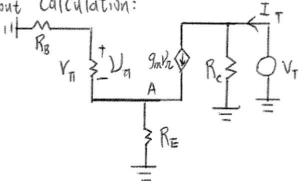
$$V_A = g_m V_{\pi} (R_E \parallel R_B + R_{\pi}) \quad (1)$$
