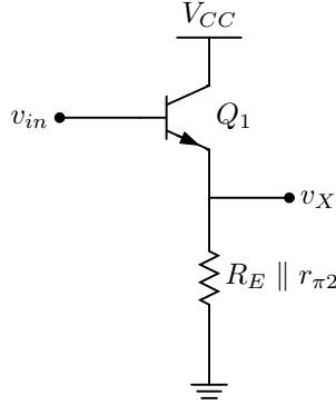
$$\frac{v_X}{v_{in}} = \frac{R_E \parallel r_{\pi 2} \parallel r_{o1}}{\frac{1}{g_{m1}} + R_E \parallel r_{\pi 2} \parallel r_{o1}}$$
