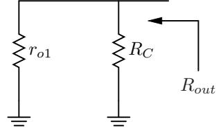
$$R_{out} = [R_C \parallel r_{o1}]$$
