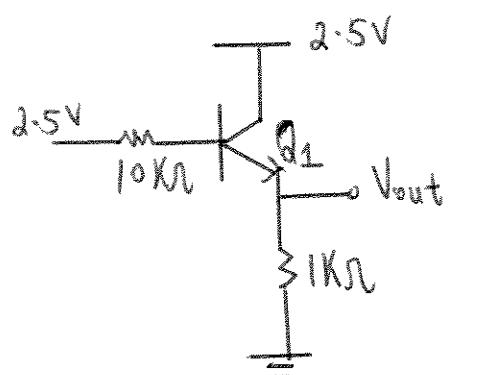
$$I_c = \beta \left( \frac{2.5 - (V_{BE} + \frac{I_c}{\alpha} 1k\Omega)}{10k\Omega} \right)$$
