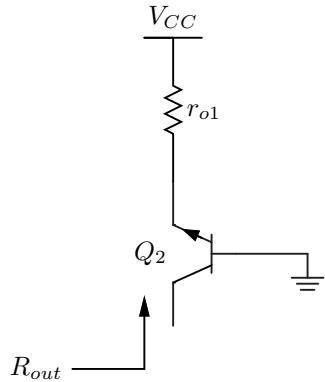
$$R_{out} = \boxed{r_{o2} + (1 + g_{m2}r_{o2}) (r_{\pi 2} \parallel r_{o1})}$$
