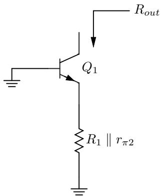
$$R_{out} = \boxed{r_{o1} + (1 + g_{m1}r_{o1}) (r_{\pi 1} \parallel R_1 \parallel r_{\pi 2})}$$
