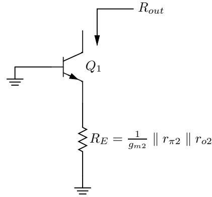
$$R_{out} = \left[ r_{o1} + (1 + g_{m1}r_{o1}) \left( r_{\pi1} \parallel \frac{1}{g_{m2}} \parallel r_{\pi2} \parallel r_{o2} \right) \right]$$
