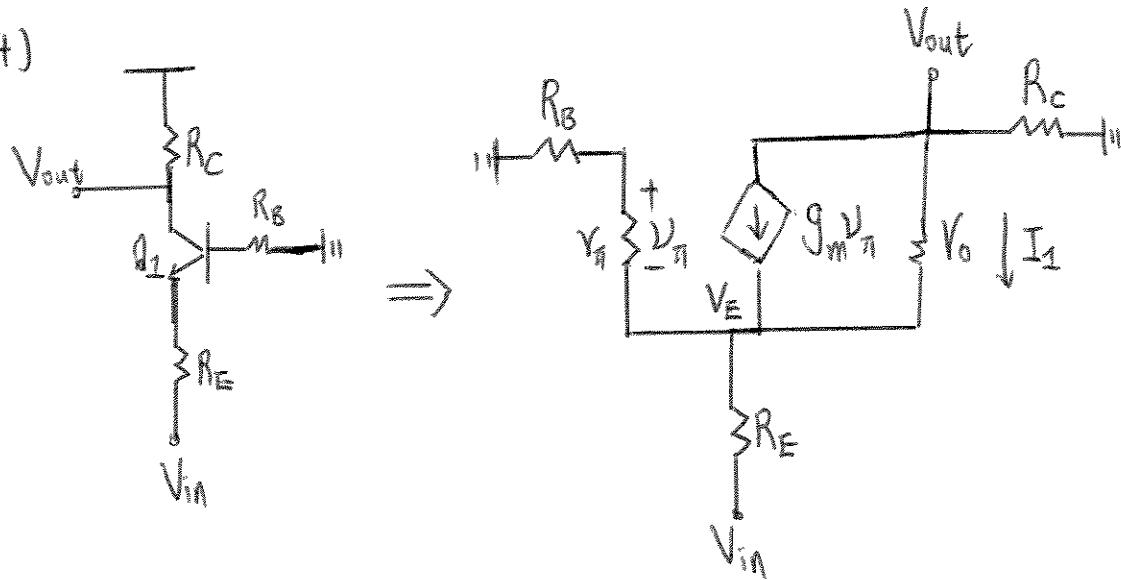
$$V_{out} = -(I_1 + g_m V_\pi) R_C, \quad I_1 = \frac{V_{out} - V_E}{R_o}$$
