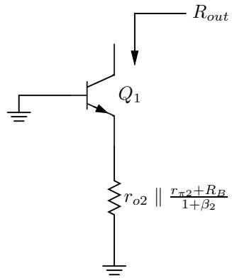
$$R_{out} = \boxed{r_{o1} + (1 + g_{m1}r_{o1}) \left( r_{\pi1} \parallel r_{o2} \parallel \frac{r_{\pi2} + R_B}{1 + \beta_2} \right)}$$
