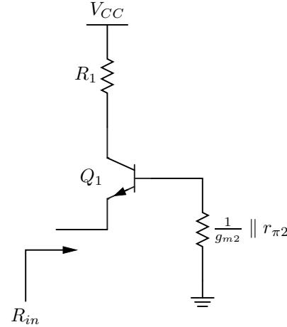
$$R_{in} = \boxed{\frac{r_{\pi 1} + \frac{1}{g_{m2}} \parallel r_{\pi 2}}{1 + \beta_1}}$$
