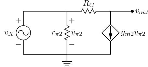
$$\frac{v_X - v_{out}}{R_C} = g_{m2} v_{\pi 2}$$
