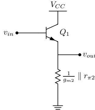
$$A_v = \boxed{\frac{\frac{1}{g_{m2}} \parallel r_{\pi2}}{\frac{1}{g_{m1}} + \frac{1}{g_{m2}} \parallel r_{\pi2}}}$$
