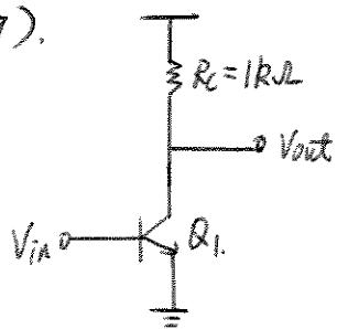
$$I_c = I_s \exp\left(\frac{V_{BE}}{2V_T}\right)$$
